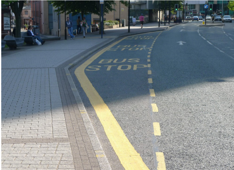
Figure 6.51 Bus pull-up zone
