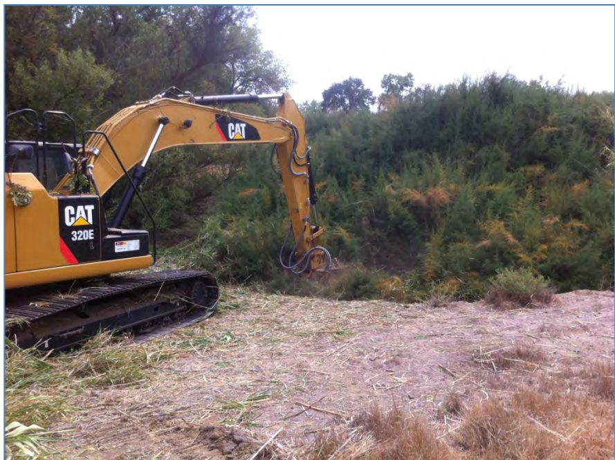
Figure 2 - excavator with special attachment chopping Tamarisk
