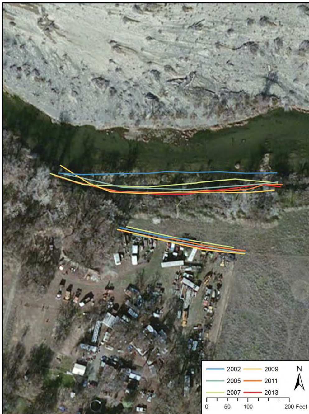
Figure 5: Digitized features used to measure the distance between the edge of the vehicle boneyard and the right bank of Cache Creek from 2002 through 2013.
