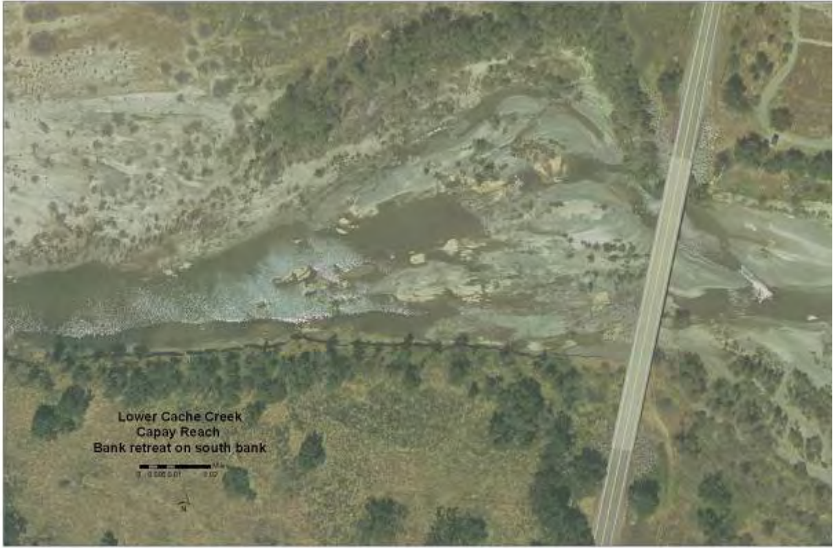
Figure 23 b Capay Reach detail of bank retreat on the south bank near Capay Bridge
