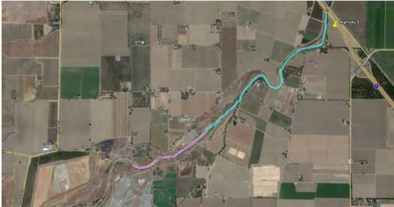
Figure 5 Areas of complete and partial flooding in the vicinity of Huff's corner (HEC-RAS)
