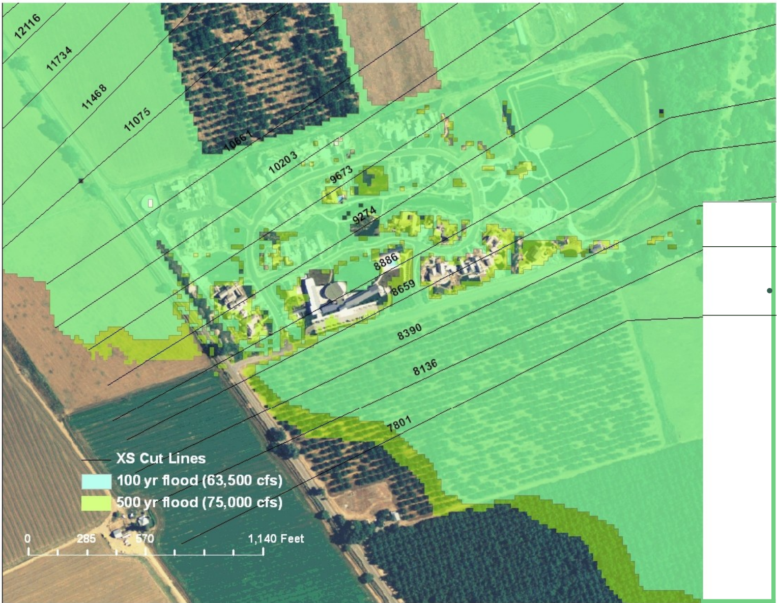
Figure 5 Flood inundation map 100 and 500 year recurrence interval flows compared (transparent overlay map colors appear distorted)
