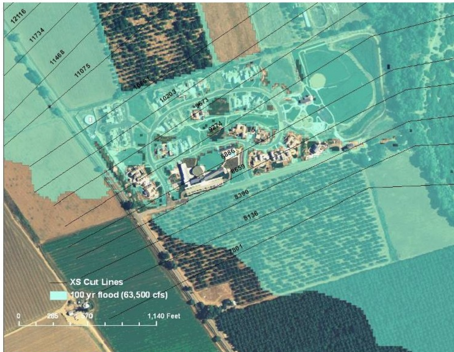
Figure 13 100-year flood inundation level in the vicinity of the Rancharia
