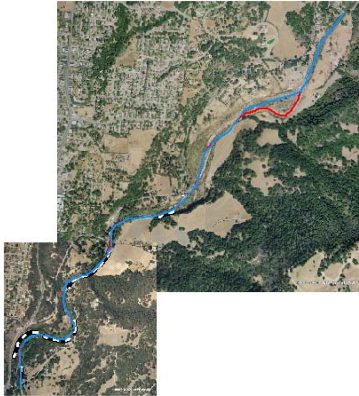
Figure 2. The entire study reach with bank restraints (black and white checked), the 2006 channel centerline including the pilot channel through the Whitman property (blue channel ), and the channel centerline if it were relocated to the pre-2005 high-flow channel (red).
